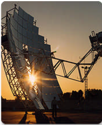
A 25-kilowatt Dish Stirling System catches its last rays of light at the end of the day. Credit: Stirling Energy Systems
